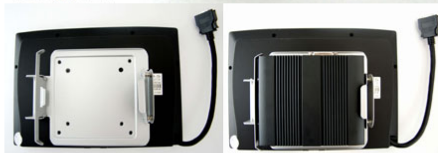
Example : QBOX mounted on CTF840-SH TFT display
